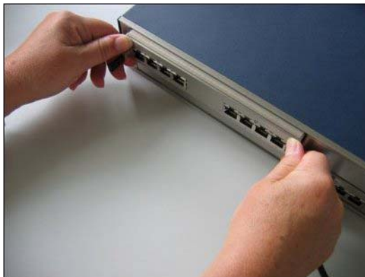
Figure: OpenScape Office MX system box – Installing a gateway module
