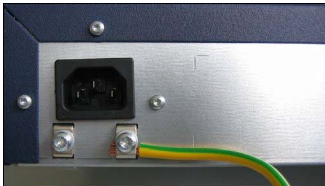
Figure: OpenScape Office MX system box – Ground wire connection
