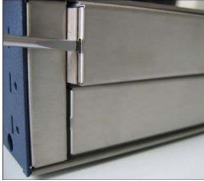
Figure: OpenScape Office MX system box – Removing a slot cover
