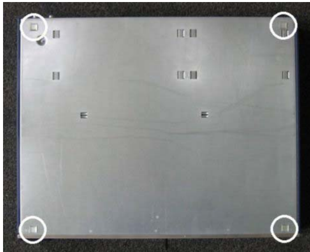
Figure: OpenScape Office MX system box – Bottom of case with mounted rubber feet
